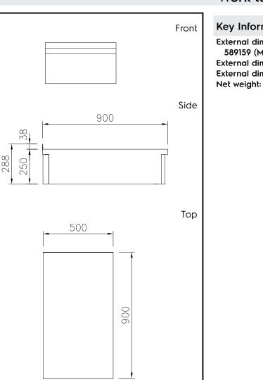
External dimensions, Width: 589159 (MCNABBEOOO) 500 mm External dimensions, Depth: 900 mm External dimensions, Height: 250 mm 23 kg
